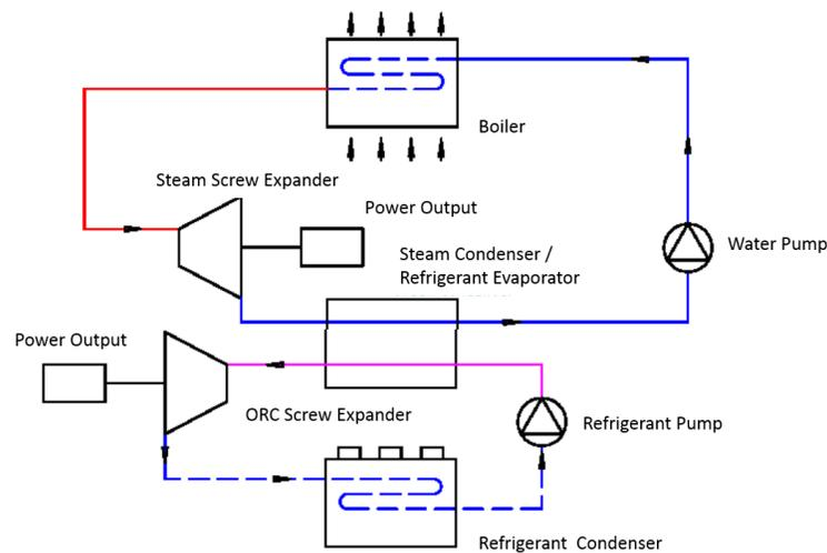
**Fig. 1:** cascaded steam and organic Rankine cycles
